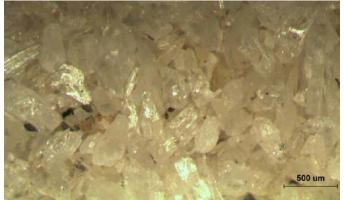
Figure 1. Spodumene grains (Image from SGS Lakefield).
